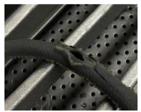
During one test in a noisy grit blast booth, the air flow was found to be below the requirement of the CSA standard. The unit had been tested many times before and always had adequate airflow. A quick inspection found the hose had a rather large hole in it. Who know how long the system had not been providing sufficient airflow to the worker? Replacing the hose was an easy fix.
