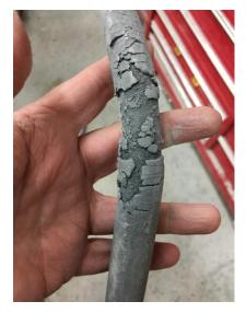
Here is a picture of a hose found in use in a workplace. The hose shows significant degradation over time. Its ability to resist chemical permeation is questionable at best.
