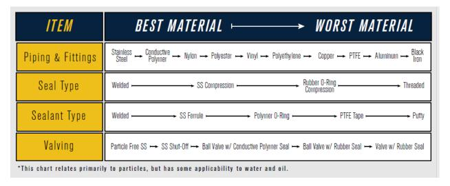
The information is provided by a lab that specializes in testing compressed air samples. The recommendations are based on laser-particle counter and general industrial experience.
