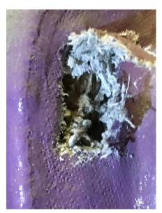
The image below would be a Medium Damage. The damage goes all the way through the outer canvas layer and damaged asbestos is exposed. However, the area is quite small. This is more of a puncture and a limited amount (less than 2 square inches) of ACM is damaged.
