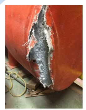
This is a second example of Severe Damage. The end of the structure has come apart exposing a significant amount of ACM. The ACM inside is damaged AND there is debris visible on the floor (right hand image.
