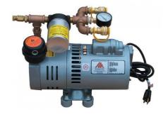
Most ambient air pumps are electrical in nature. The come in sizes of ¾ HP to 2 HP. They provide a low pressure (<15 psi) output. Because of their modest size, they have limited air flow so the number of workers on a pump is limited. The number of workers depends on whether they are using loose fitting hoods or tight-fitting facepieces.
