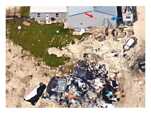
Intake Located Near Combustion Source
